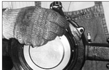
Figure 8 – Shows how to measure the gap between the body seat pocket ID and the disc OD.
