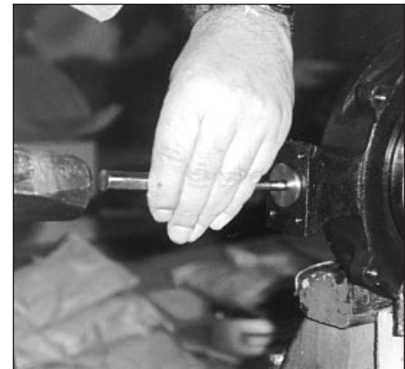
Figure 9 – Shows how to lock the tapered pin into position.
