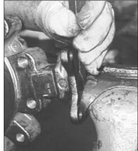
Figure 4 – Shows how the upper stem is removed from the upper disc hub.
