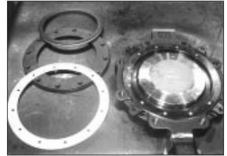
Figure 11 – Shows dead-end service seat assembly.
