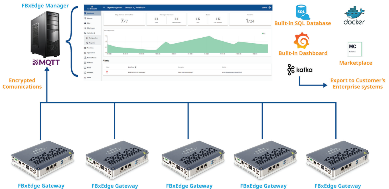
Figure 9: FBxEdge Manager enables FBxEdge users to leverage powerful central management capabilities, including bulk deployment of tags, applications, and remote upgrades.
