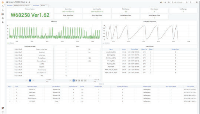
Figure 6: FBxEdge users have access to Grafana, an open-source visualization application, to generate charts, graphs and more.
