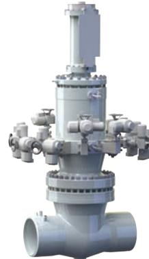
Parallel slide gate valves have a mechanical coupling that keeps the valve open in the event of zero system pressure.
