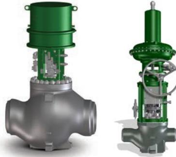
Globe straight or angle style valves with live loaded graphite packing and seismic bonnet on a designated piston or air operated actuator. Installed in EPR and AP1000 nuclear plants.
