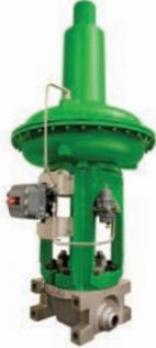
Globe straight or angle style valves with live loaded graphite packing and a seismic bonnet on a designated piston or air operated actuator. Installed in EPR and AP1000 Nuclear plants.
