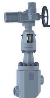
Bellows-sealed, Z-form forged body, high quality material, cobalt free hard facing at seat, disc and guiding surfaces. Different control characteristics available, permanent flow over throttle in the valve disc to keep the spray lines and the volume compensation line at a given temperature.
