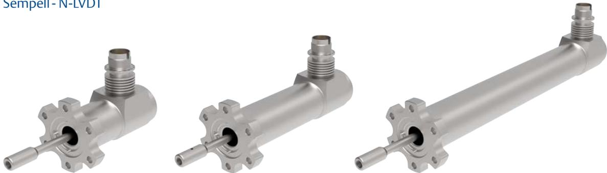
Sempell N-LVDT is a linear valve position transmitter. This instrument is mounted on a linear sliding stem valves and it is designed for precise measurement of linear displacement or position. These transducers are built to be highly robust, with an inherently frictionless and infinite lifecycle design.
