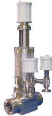
Pilot operated gate valves with mechanical coupling to keep the valves open in the absence of system pressure and pneumatic actuator for operation in absence of system media.
