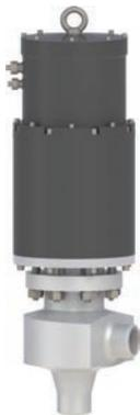
Solenoid-controlled spray valves ensuring opening or closing in accordance with the coolant pressure, closed during normal operation. The valve has a small borehole in the valve disc to keep the spray lines and the volume compensation line at a given temperature with a continuous flow rate.
