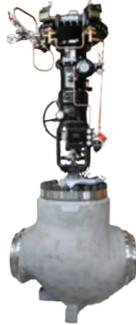
This globe valve with EUT design is a single port control valve, balanced valve plug, cage guiding and metal to metal seating for all applications over a wide range of process pressure drops and temperature.
