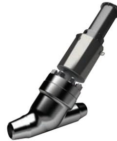
Emerson uses third party technology for a modulating solenoid valve in response to the plant's flow control command. This technology consists of a pilot-operated solenoid valve, a LVDT for position indication, and a proprietary electronic positioner to create a closed feedback loop. It is particularly well suited where a pneumatic supply, required for traditional control valves, cannot be provided.
