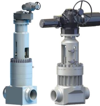
Designed for steam and water circuits operable at guillotine pipe-break and after electric actuator switch-off failure. Split wedge design delivers superior leak tightness.
