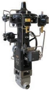
Valves with live-loaded packing and seismic design. They can be equipped either with manual air-operated or electric actuators. Installed in most Generation 2 and 3 nuclear power stations, this design may be used in general high pressure/temperature fluid control applications with multiple trim combinations.
