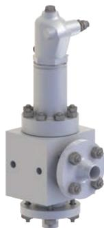
PSE valves are used specifically in liquid applications where a proportional characteristic is required. Above set pressure, these valves open steadily with increasing pressure ensuring only the necessary capacity is relieved during opening.
