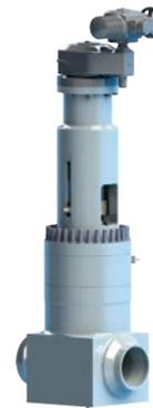
Designed for steam and water circuits, these valves operate in the event of a guillotine pipe-break or after an electric actuator switch-off failure. Their split wedge, limit switch control design provides superior leak tightness, precise wedge guiding and D-shaped wedges to avoid tilting.
