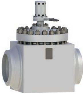
A swing check valve suitable for steam and water with a one-piece block-design. A special retaining ring assembly enables precise flap positioning. The lack of a shaft duct excludes leakages to the outside and ensures the function is not impaired by friction in the glands.
