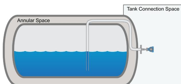
Figure 3. Horizontal C-tank with a bended still pipe entering from the tank connection space
