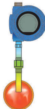
Figure 3-99: Temperature Propagating from Pipe to Transmitter
