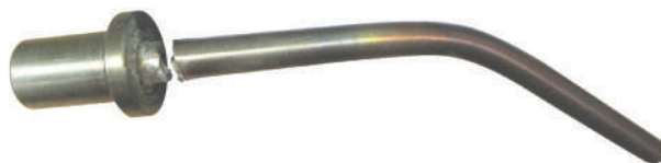
Figure 3-91: Example of a Thermowell Failure
