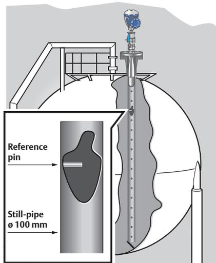
Figure 7.1: Level measurement in a spherical gas tank using a still-pipe with reference pins.
