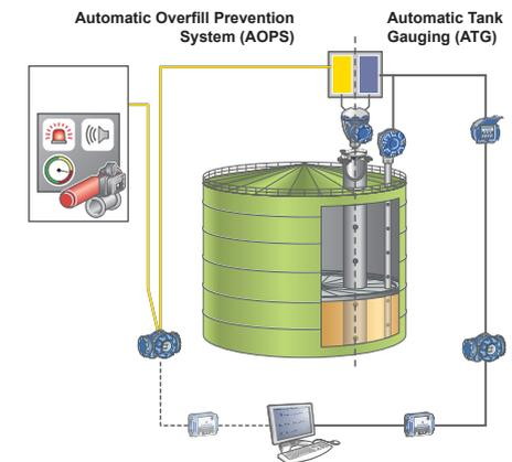
Figure 10.11: System overview for 2-in-1 radar level measurement.
