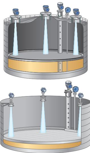
Figure 1.7: Up to six non-contacting level instruments are placed either at the tank shell or on top of the outer roof. Roof tilt is tracked by comparing the distance between each device and the floating roof.
