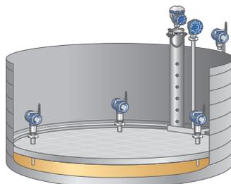
Figure 1.8: Up to six guided wave level transmitters can be installed directly on the floating roof, with rigid probes penetrating through the roof and into the liquid below. Roof tilt is tracked by comparing the distance from the floating roof down to the product surface. With one or two extra transmitters one can also detect if the roof drain gets plugged or if there is any hydrocarbon on the tank roof.
