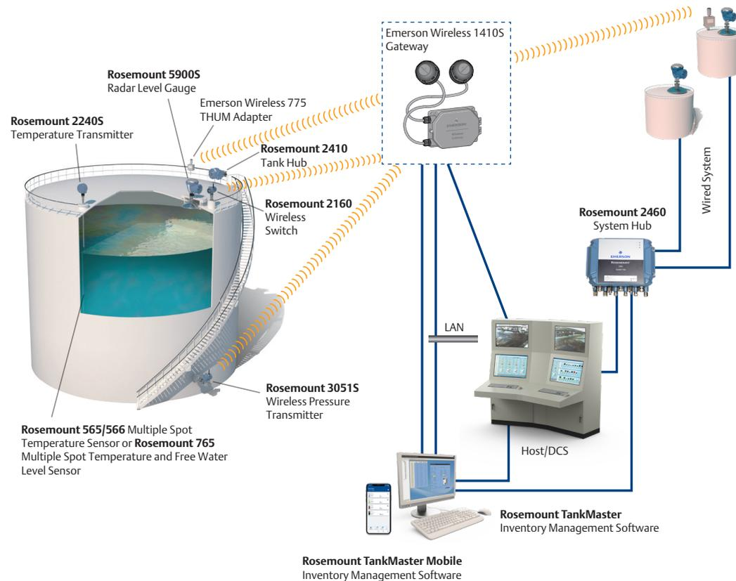
A wireless tank gauging solution designed specifically for every customers' bulk liquid storage plant maximizes safety and operational performance.
