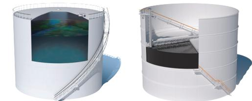
Figure 1.2: Fixed roof and floating roof tanks.
