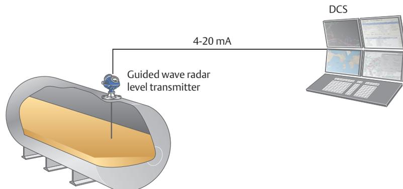
Figure 5.4: Typical process level transmitter architecture.
