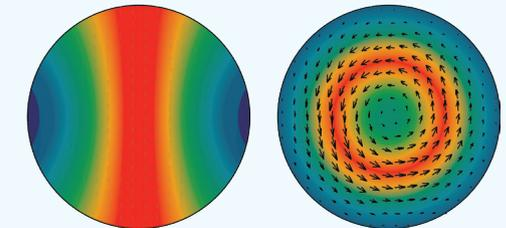
Figure 2.17: Low loss H01 mode visualized.
