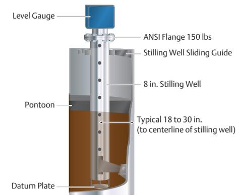
Figure 3.3: Still-pipe attached to the tank wall.
