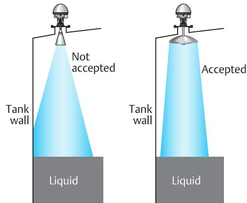
Figure 2.15: Radar gauges with wide beam (small antenna) and narrow beam (large antenna).
