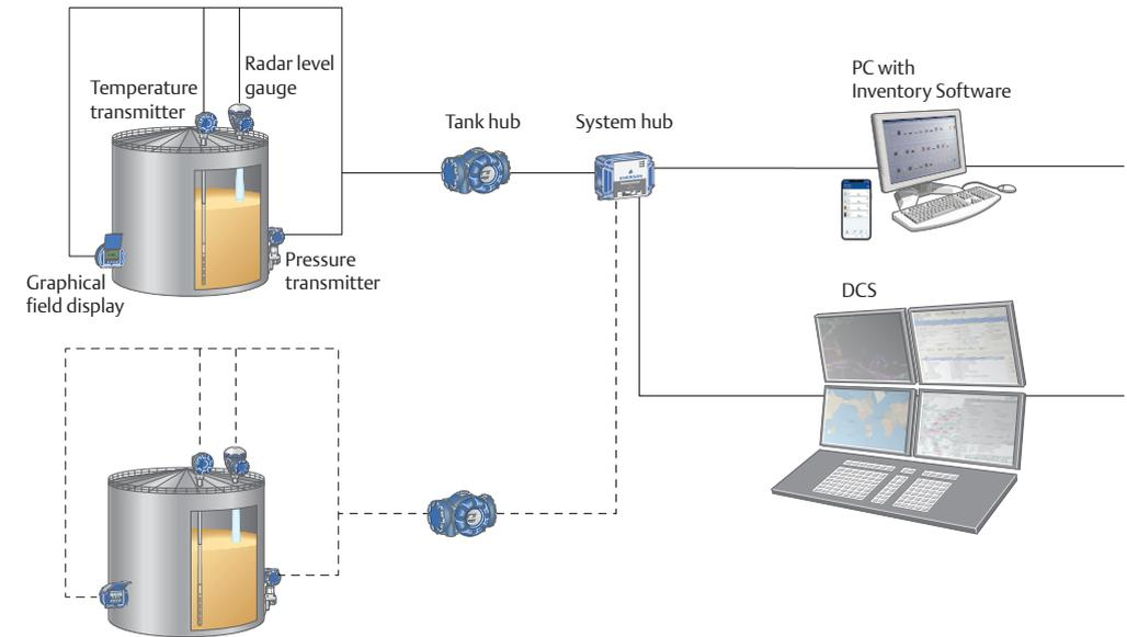
Figure 5.5: Typical tank gauging system architecture.
