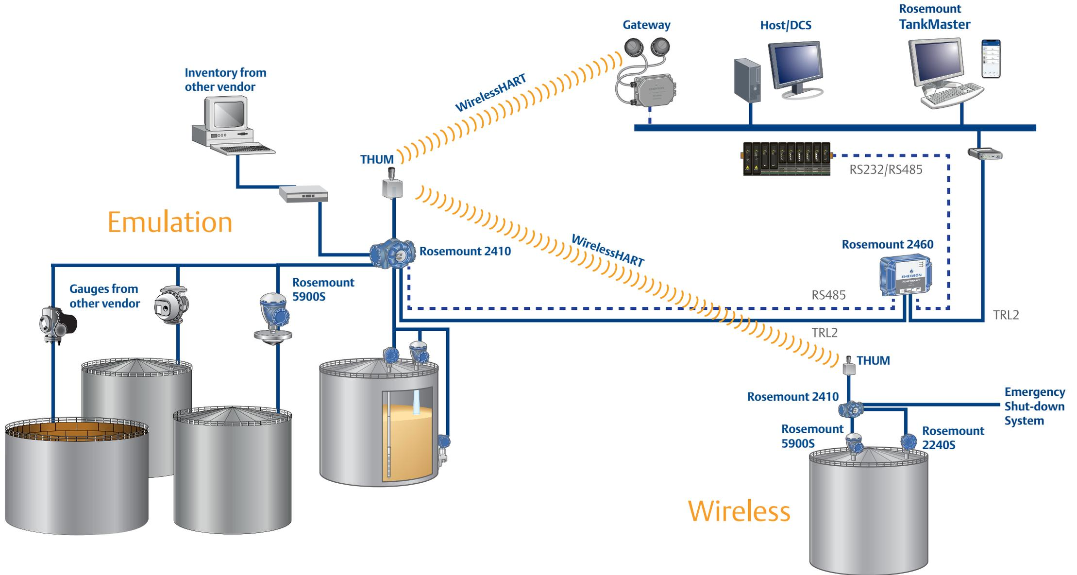
Adding a wireless network can bridge the gaps of the legacy bus system. By doing this, the user can get an additional communication channel for gauging, configuration and diagnostics.
