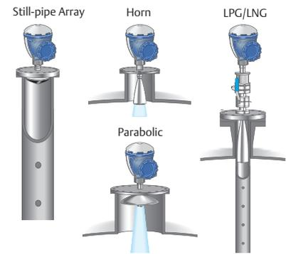
Rosemount 5900C Radar Level Gauge
