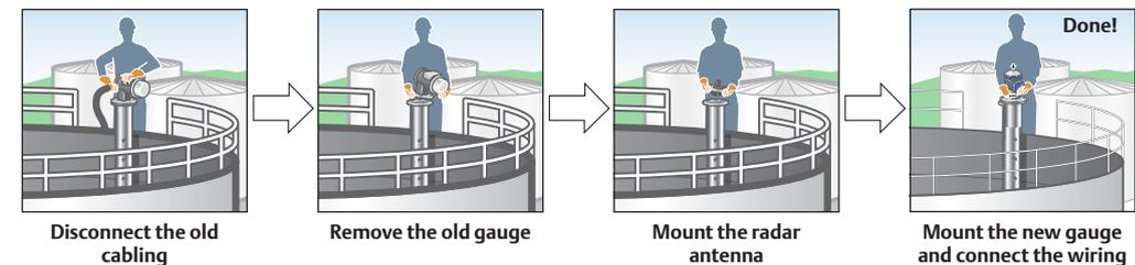
Figure 9.6: With gauge emulation, a tank by tank upgrade is easy.
