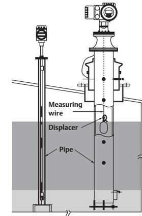
Figure 2.7: Servo gauge and temperature sensor measuring inside still-pipes.
