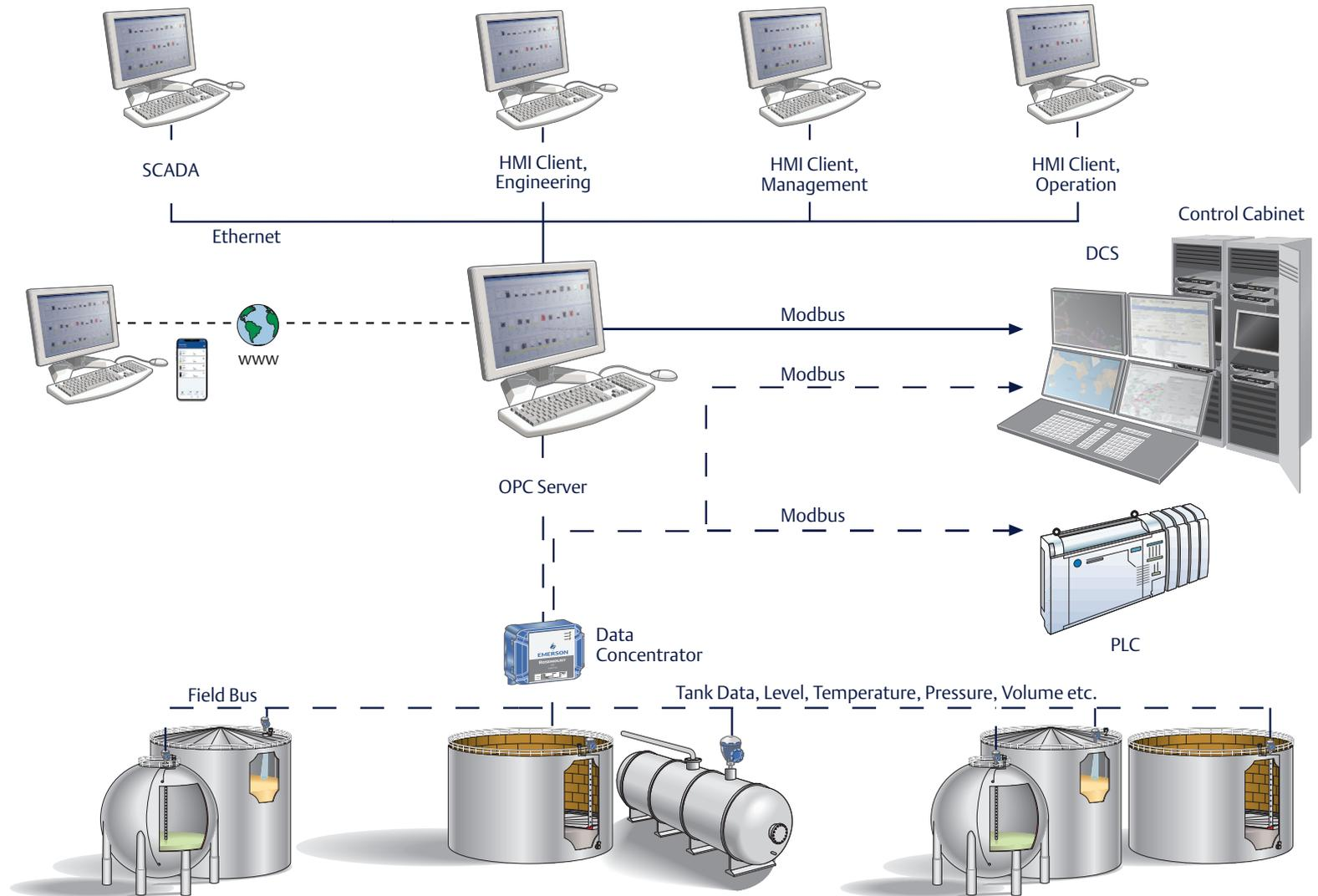
Figure 9.1: Modern tank gauging system architecture.
