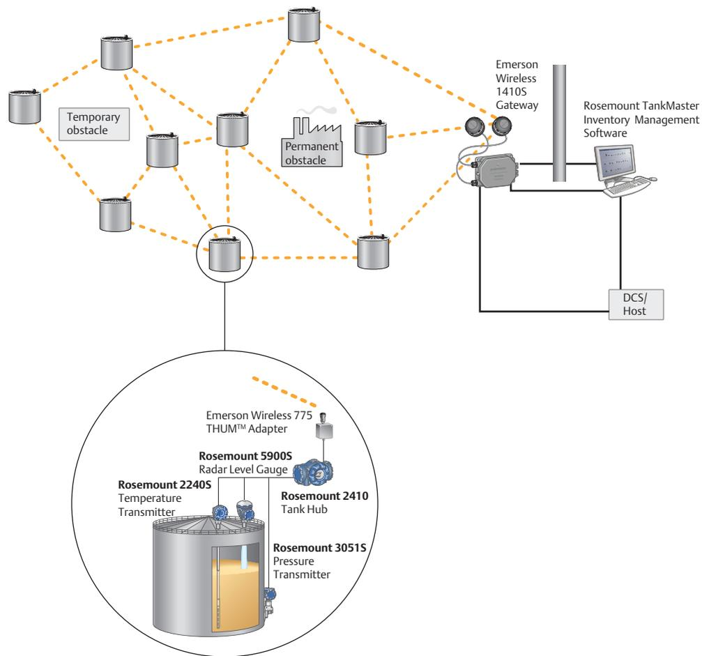
All wireless devices communicate with the host system through the wireless gateway. A Rosemount Tank Gauging System may consist of both wired and wireless networks.
