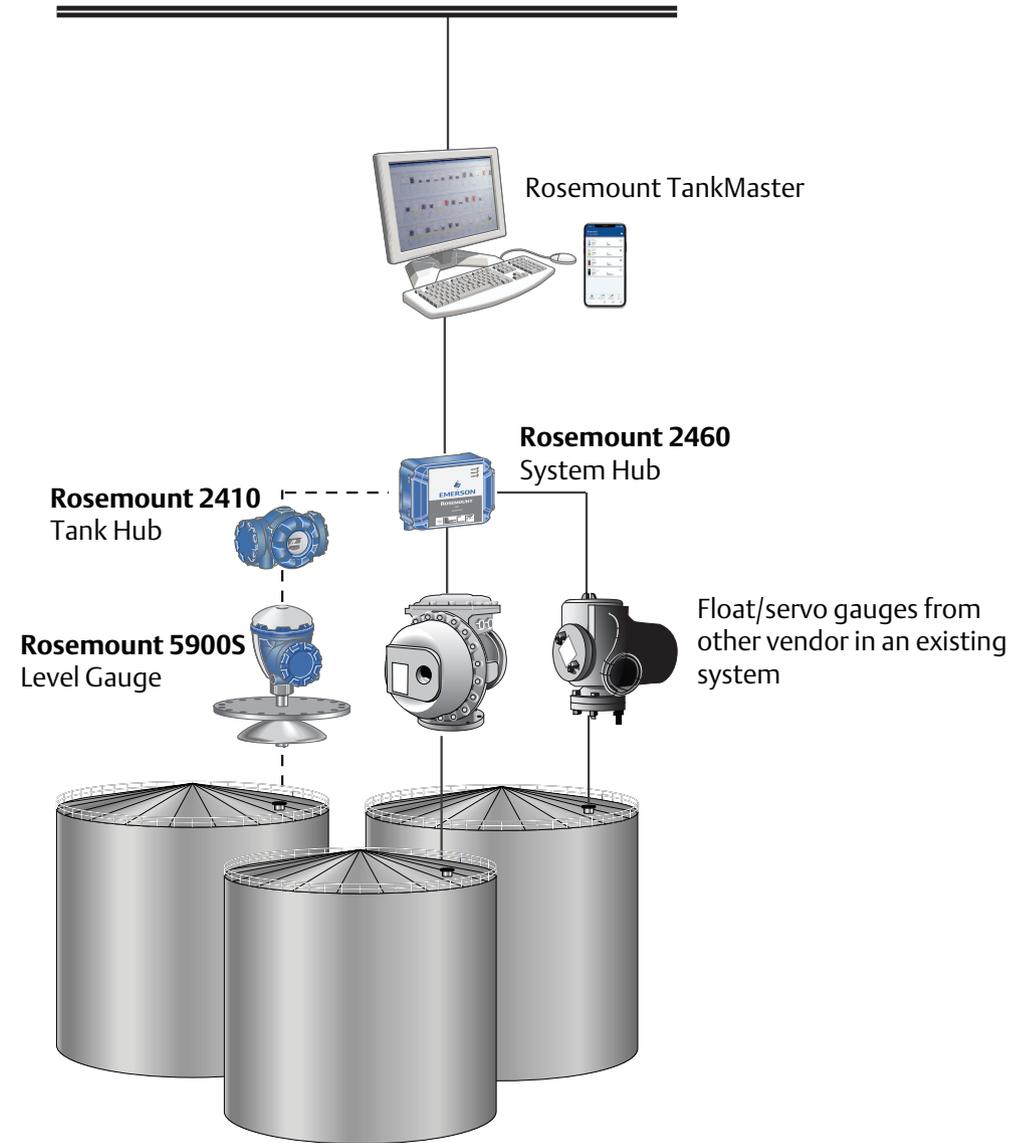
Replacing old tank monitoring software with TankMaster.
