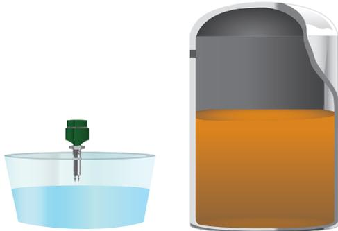
Figure 10.12: Traditional approach to proof-testing - bucket testing.
