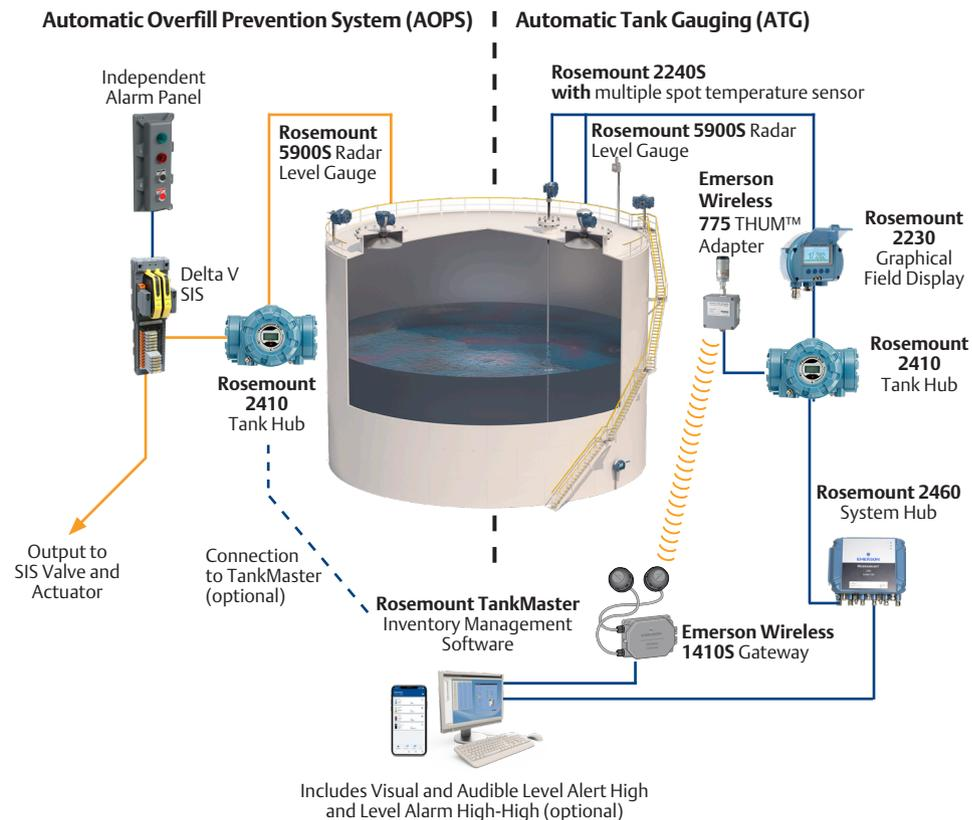
Example of a modern approach to overfill prevention, incorporating an automatic overfill prevention system based on continuous radar level measurement.
