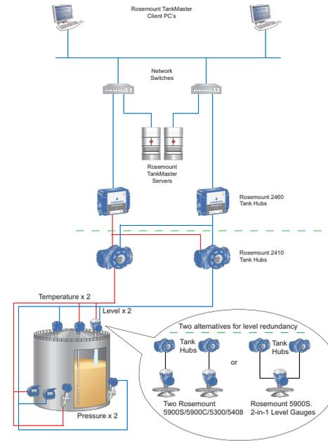
Figure 9.4: Different layers of redundancy: Tank unit redundancy and field communication unit redundancy combined with redundant data servers and operator stations.
