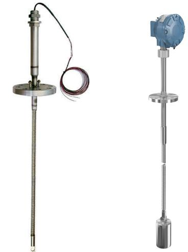
Figure 6.2: Left - Multi-spot temperature sensor with Pt100 elements and corrosion resistant metallic sheath. Right - Complete temperature measuring assembly with transmitter, sensor, optional water level sensor and anchor weight.
