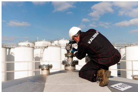
Figure 2.2: Hand gauging with a dipping tape.
