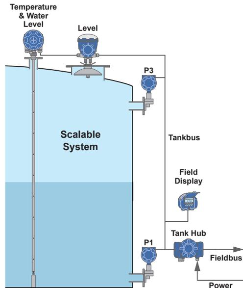
Figure 9.2: Intrinsically safe field bus providing power and communication to the tank units.
