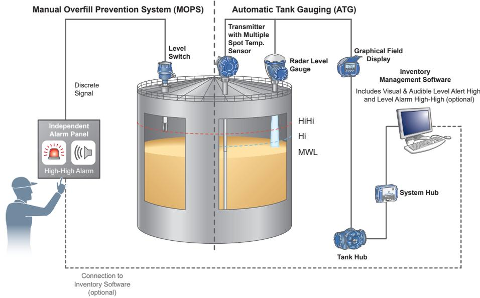
Figure 10.8: The traditional (obsolete) approach to overfill prevention - manual systems based on point-level measurement.
