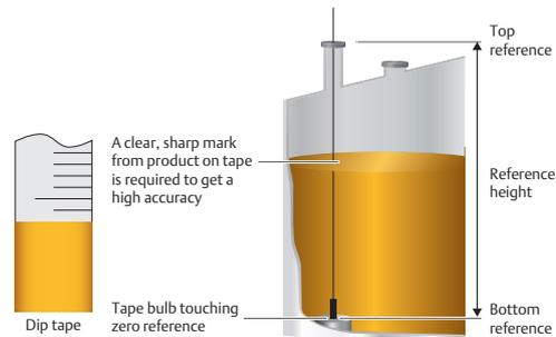
Figure 2.4: Manual level measurement definitions.
