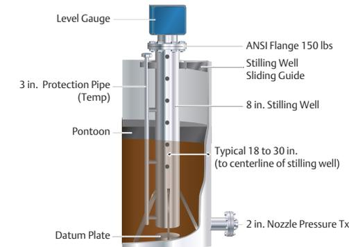
Figure 3.2: Still-pipe attached to the tank bottom.
