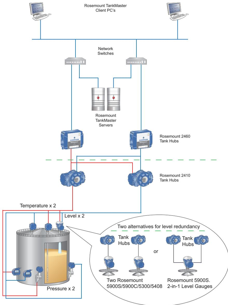
A fully redundant tank gauging system with four levels of redundancy: Tank unit redundancy and field communication unit redundancy combined with redundant data servers and redundant operator stations.
