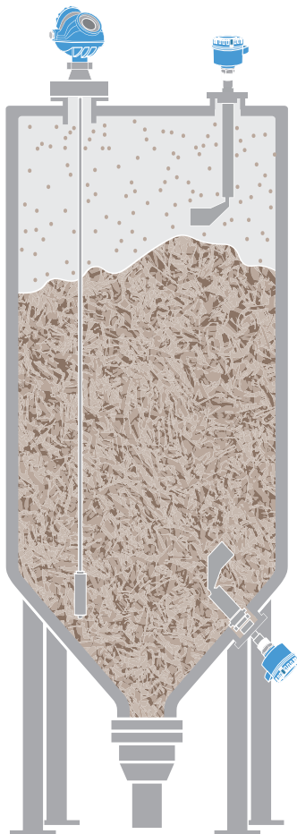
Figure 5.2.14: Corn surge bin with guided wave radar and paddle switches
