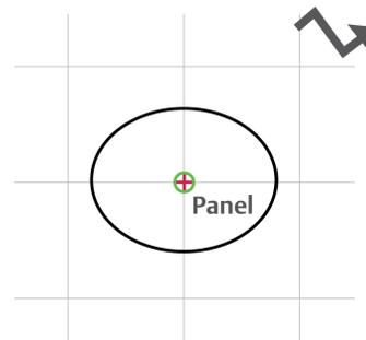
*WirelessHART* devices can be connected to a *WirelessHART* Gateway using the User Defined Field. This type of drawing does not show the path through the *WirelessHART* network, but does show the relationship of the *WirelessHART* device and the *WirelessHART* Gateway; Figure 13-7 is an example from the ISA-5.1.
