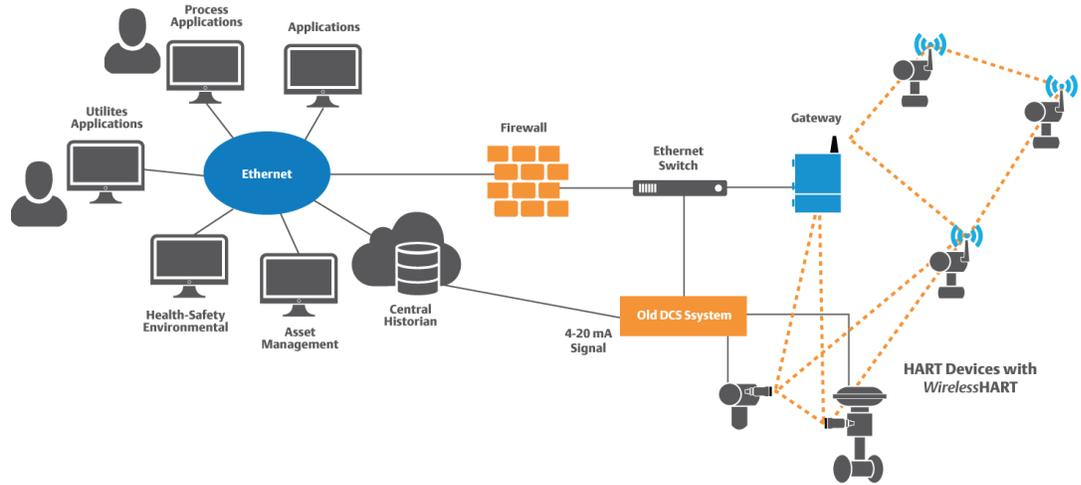
A key output from working with host system administrators is an integration strategy to incorporate a plant-wide wireless infrastructure. If doing a small application, a key output is the physical locations of where to connect the Gateways. These will be needed for the network design process.
