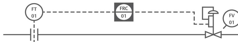
B.9.4 Shared Display, Shared Control Instrumentation with Diagnostic and Calibration Bus on Field Wiring:
