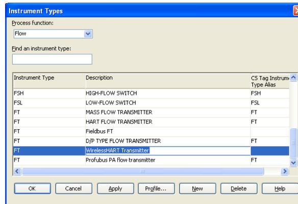
The first step is to create a new device with a new description. In this example, a *WirelessHART* flow transmitter is created. Please note that if the device will be specified as a wired HART device with a *WirelessHART* adapter, no new instrument types are necessary
