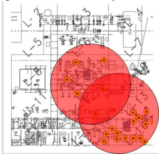
If a wireless device requires update rates faster than two seconds or is used for control and does not meet the “Rule of Maximum Distance”, consider adding a Gateway as shown in [Figure 6-8](#) or moving the existing Gateway closer to the wireless device. If the process control loop is tolerant of latency, or if it was previously a form of manual control, it may be acceptable to have devices further from the Gateway.
