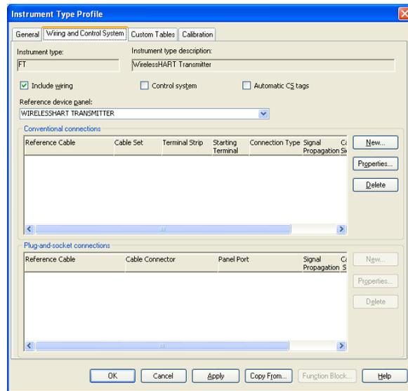
Check the box to include the wiring. If this box is not checked when SPI generates loop drawings, the device cannot be added to loop drawings. This also allows for flexibility for different wiring configurations, to be defined elsewhere. Examples include wiring *WirelessHART* adapters in series with the loop and line power for *WirelessHART* devices. This process should be repeated for each unique *WirelessHART* instrument type.
