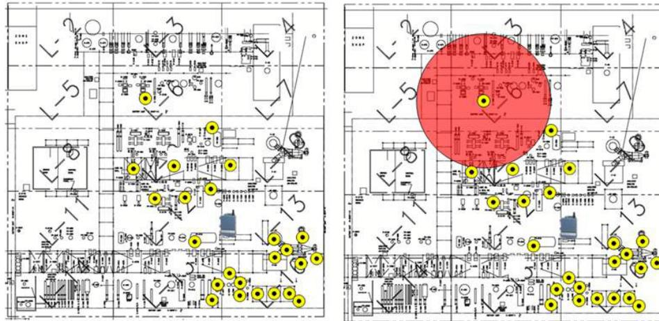
The self-organizing mesh technology allows for more *WirelessHART* field devices to be added to a network for the purposes of automation, and provides the means for simple design correction to also exist. A stress failure can be fortified by moving the Gateway location, adding a new Gateway to segment the network, adding more devices or adding repeaters.
