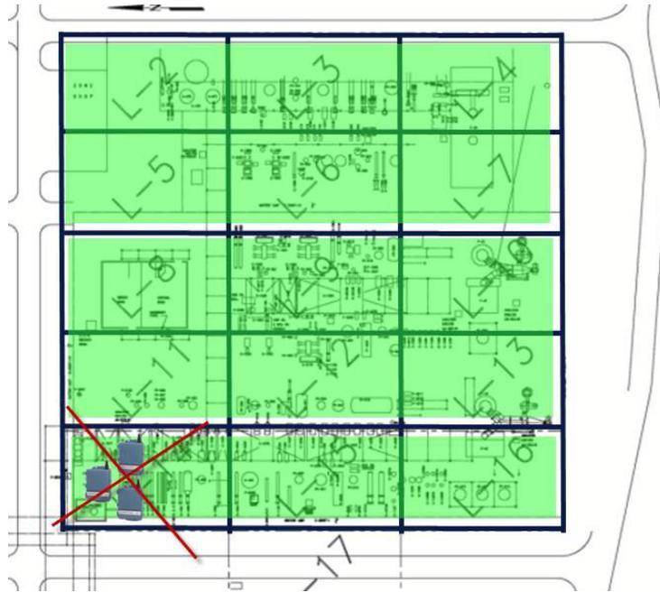
Do not place all Gateways in the same location just because connecting into the host system is convenient. The next section on network design will show that this is inefficient and can lead to unreliable networks in the long term. The Gateway should be centralized to the field network to maximize the number of connections to wireless devices.
