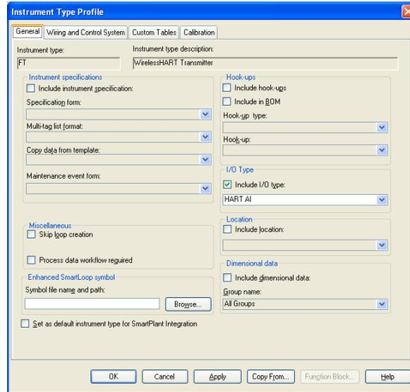
Nothing needs to change on the general tab. Be sure to leverage that the device is a HART AI or a HART AO so that all of the basic parameters of HART apply. Manage the wiring, or lack of wiring separately. The fact that *WirelessHART* is based on HART allows leverage of these pre-defined variables.
