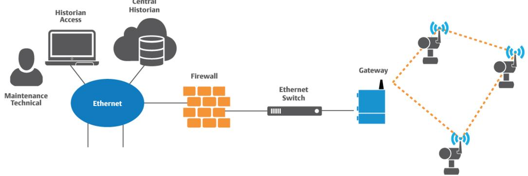
For *WirelessHART* networks that support users in different roles, the potential exists for each end user to have their own application for collecting and analyzing data. For users who manually collect data, *WirelessHART* provides the missing piece to automation.
