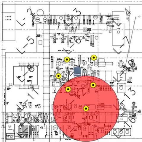
3. “Rule of Percentages” – Every *WirelessHART* network with greater than five devices should have a minimum of 25 percent of devices within effective range of the Gateway to ensure proper bandwidth and eliminate pinch points. *WirelessHART* networks can work with as little as 10 percent, and actual implementation may yield less than 25 percent, but experience shows this is a practical number. Example, a 100 device network implies 25 within effective range of the Gateway.
