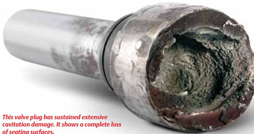
*This valve plug has sustained extensive cavitation damage. It shows a complete loss of seating surfaces.*
