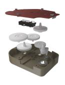
Simple and robust absolute position encoder sensor with high reliability and accuracy, which allows for position detection even when mains and back-up power are lost. Position accuracy is within 0.1% of true position, and position is recordable up to 8,580 full rotary cycles of the actuator's output shaft.
