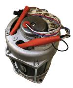
**Speed sensor** on the motor is equipped with a microprocessor to accurately record torque data. A thermostat also resides on top of the motor, which trips the motor if it over-heats (caused by the actuator being pushed beyond its rated torque).
