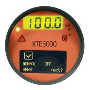
Intuitive user interface requires minimal training to use. The viewing glass is resistant to discoloration from strong sunlight, and the transflective LCD and OLED displays are easy to read in even the brightest or darkest environments.
