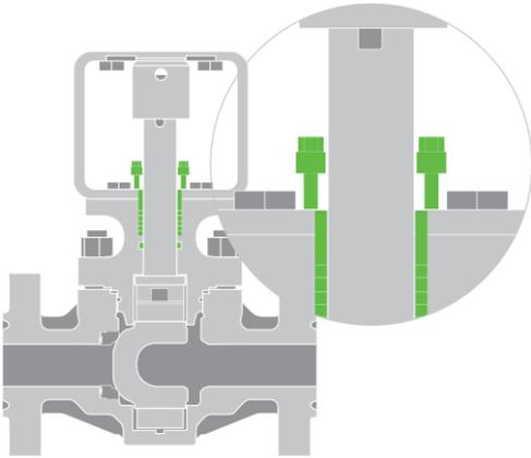
**Be confident that your valves meet regulatory emissions** levels on a long-term basis without the need for maintenance or intervention. The true quarter turn design and advanced high temperature, live loaded packing is self-adjusting for long-lived, ultra-low emissions.
