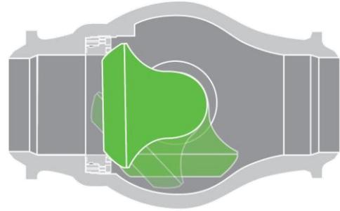
**Run your process for longer** with a double offset C-ball design that enables non rubbing rotation to eliminate wear and extend maintenance intervals. The convex to convex seat is designed to “sweep” particles off the sealing surface without damage, making it ideal for abrasive service which means low wear and long-lasting tight shutoff.
