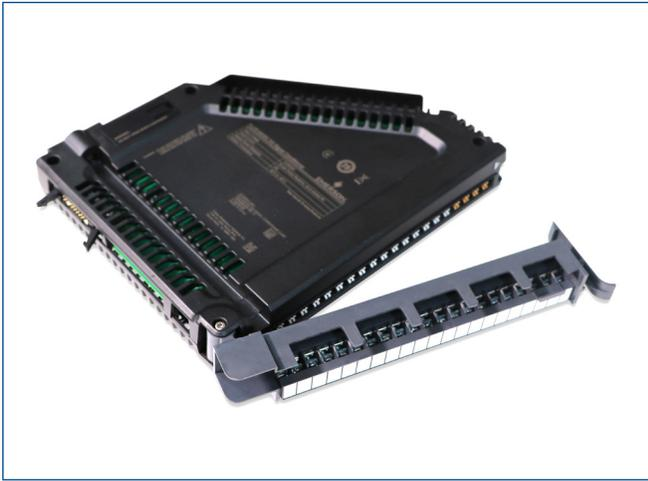
The Discrete Output (DO) 24 VDC non-isolated Signal Conditioning Card for 1771 I/O connects to the simplex or redundant M-series Plus DO, 32-Channel, 24 VDC, High-Side card by using two of the 20-pin standard Round Ribbon Cables; one for each of the two 16-channel Signal Conditioning Cards for 1771 I/O. The 21-position OEM contact 1771-WH swing-arm is removed from the OEM 16-channel, DO, 24 VDC, 1771-OBD card and placed on the 16-channel DO 24 VDC, non-isolated, Signal Conditioning Card.
