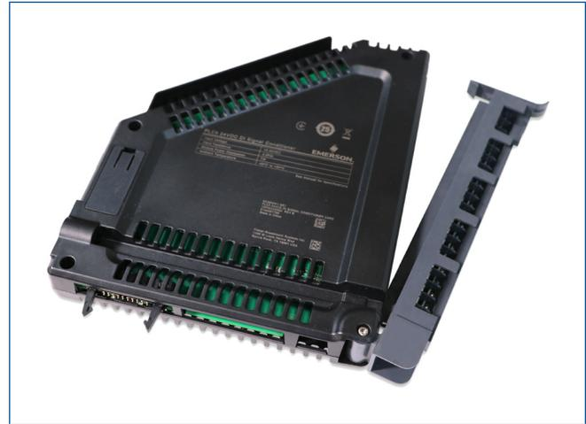
The Discrete Input (DI) 24 VDC non-isolated Signal Conditioning Card for 1771 I/O connects to the simplex or redundant M-series Plus DI, 32-Channel, 24 VDC, Dry Contact card by using two of the 20-pin standard Round Ribbon Cables; one for each of the two 16-channel Signal Conditioning Cards for 1771 I/O.
