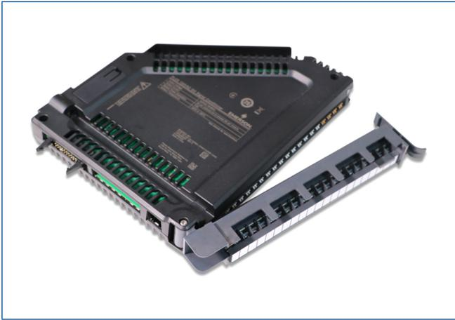
The **Discrete Output (DO) 120 VAC non-isolated Signal Conditioning Card for 1771 I/O** connects to the simplex or redundant M-series Plus DO, 32-Channel, 24 VDC, High-Side card by using two of the 20-pin standard Round Ribbon Cables; one for each of the two 16-channel Signal Conditioning Cards for 1771 I/O.
