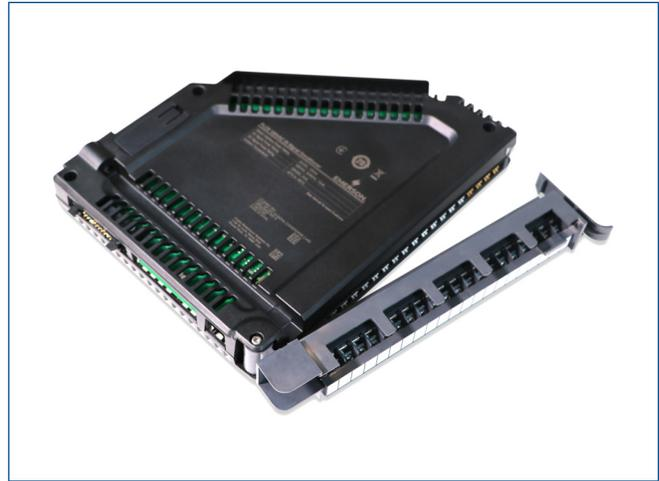
The Discrete Input (DI) 120 VAC/VDC non-isolated Signal Conditioning Card for 1771 I/O connects to the simplex or redundant M-series Plus DI, 32-Channel, 24 VDC, Dry Contact card by using two of the 20-pin standard Round Ribbon Cables; one for each of the two 16-channel Signal Conditioning Cards for 1771 I/O. The 21-position OEM contact 1771-WH swing-arm is removed from the OEM 16-channel, DI, 120 VAC/VDC, 1771-IAD card and placed on the 16-channel DI, non-isolated, Signal Conditioning Card.
