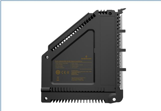
**The Discrete Input (DI) 120 VAC/VDC isolated Signal Conditioning Card** for 1771 I/O connects to the simplex or redundant M-series Plus DI, 32-Channel, 24 VDC, Dry Contact card by using two of the 20-pin standard Round Ribbon Cables; one for each of the two 16-channel Signal Conditioning Cards for 1771 I/O.
