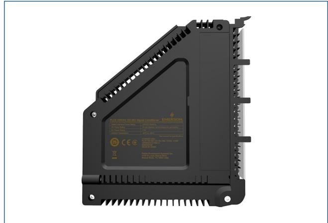
**The Discrete Output (DO) 120 VAC isolated Signal Conditioning Card** for 1771 I/O connects to the simplex or redundant M-series Plus DO, 32-Channel, 24 VDC, High-Side card by using two of the 20-pin standard Round Ribbon Cables; one for each of the two 16-channel Signal Conditioning Cards for 1771 I/O.
