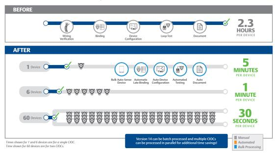
Automation and parallel processing enables commissioning to be completed in a fraction of the time per device.
