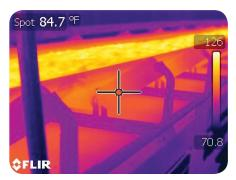
antifreeze before it enters the bunker. However, antifreeze is expensive, and may not be needed if the coal going in is warm enough. An IR camera can provide non-contact temperature measurements to resolve this issue and save cost in the long run.
