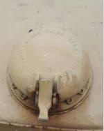
"This was a challenging solution to develop. Sensing that the lid was closed wasn't enough, we had to confirm that the hatch was properly latched, without giving a false positive. We ended up with a design that was easily installed in the field on both new and existing thief hatches, and not just something that looked good on paper."
