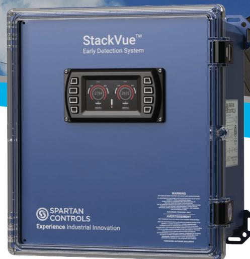
To address this need, the StackVue™ continuously monitors for the ignition of liquid hydrocarbons within the heat exchanger tube. By analyzing clean natural gas exhaust for unwanted hydrocarbons, specifically oil or a derivative of the oil gases passing in the flue stack. The combustion of another hydrocarbon can be detected and the system will provide a safety shutdown to the burner management system to ensure that there is no chance of continued fire or excessive appliance or building damage.
