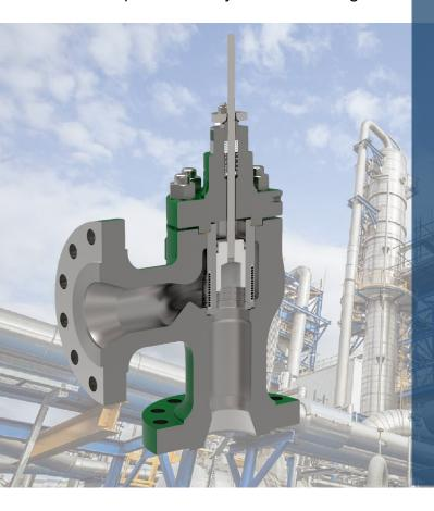
Fisher HP series control valves are singleport, high-pressure, globe- or angle-style valves with metal seats, cage guides, and push-down-to-close valve plug action.
