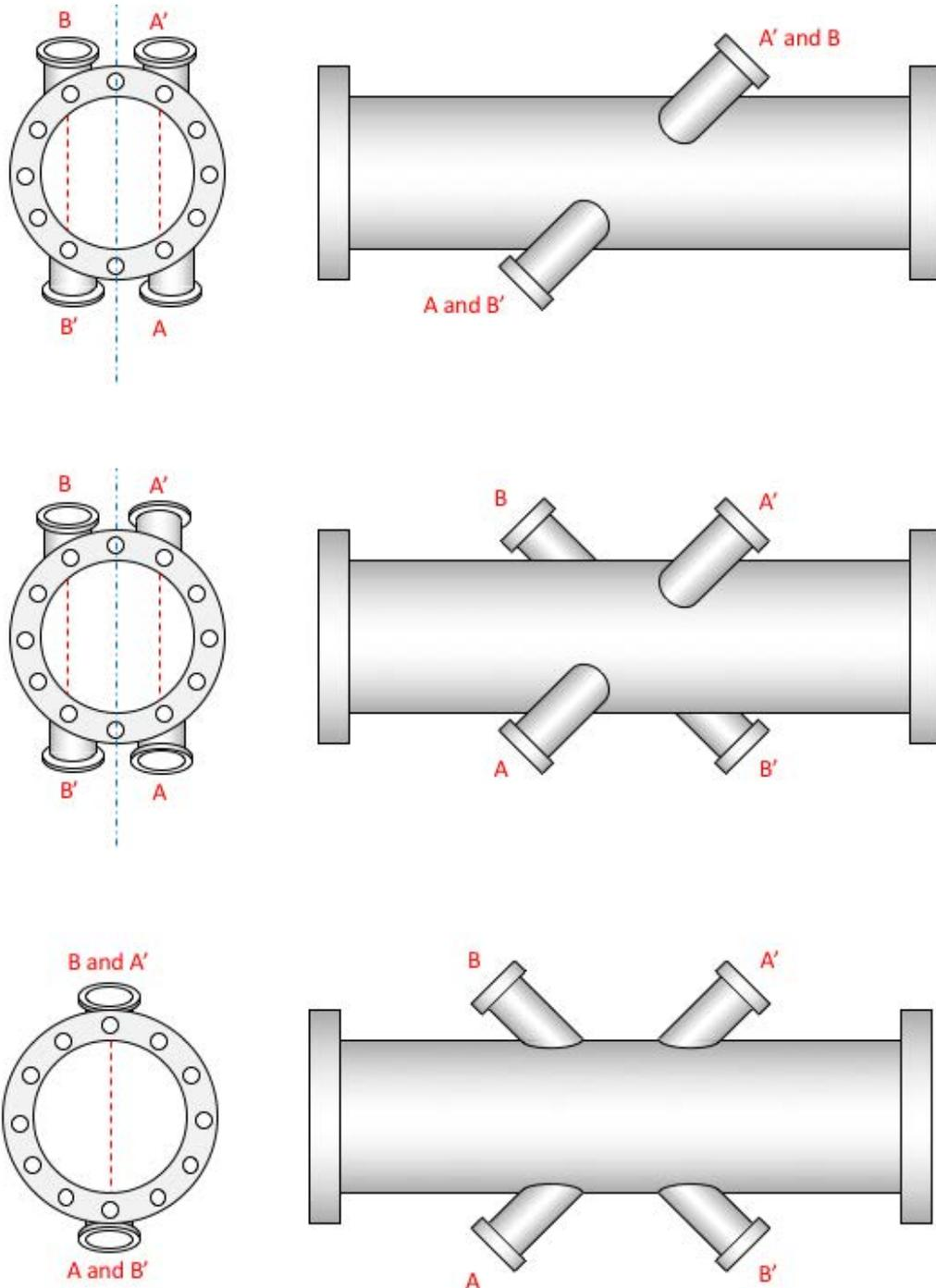
Fluenta offers a wide range of installation options for dual-path measurement.
