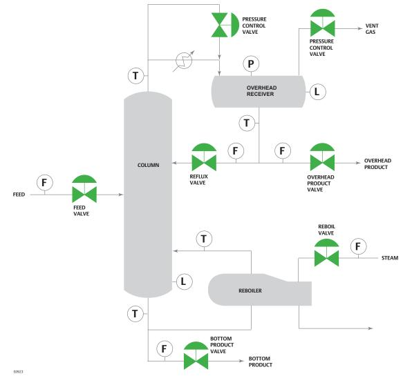
Figure 2. Distillation Column Process Flow Diagram
