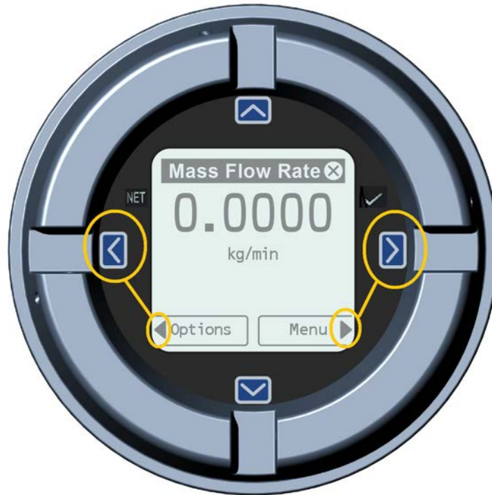
Figure 6-2: Example 2: Active arrow indicators on the transmitter display
