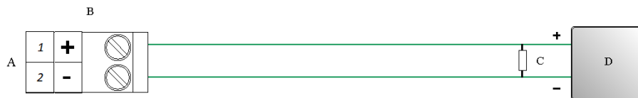
Figure 3-11: Frequency output wiring (internally powered)
