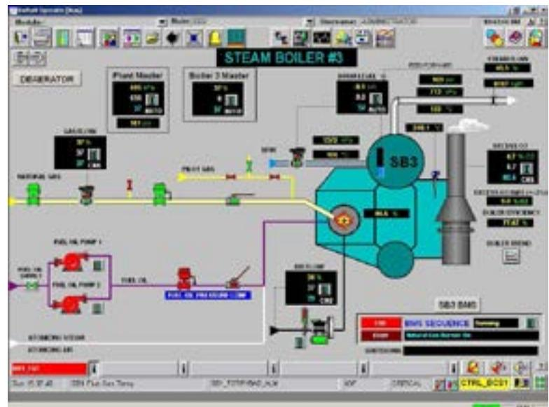
Boiler efficiency can have a big impact on plant fuel gas costs and emissions. High levels of oxygen in the stack gases indicate that the boiler is operating at suboptimal efficiency, wasting fuel, and generating excess emissions. This is typically due to:
