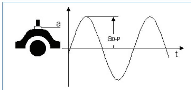
Figure 11. Bearing acceleration Peak ( $a_{0-p}$ ): 0 to Peak.
