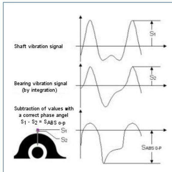
Figure 8. Absolute shaft vibration
