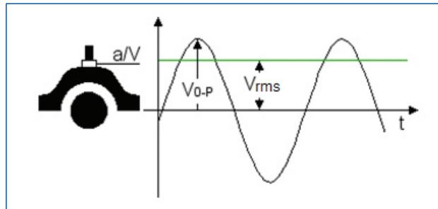
Figure 12. Bearing velocity ( $V_{rms}$ ): RMS.
