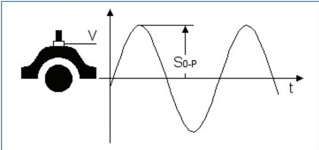
Figure 14. Bearing vibration  $S_{0-p}$ : 0 to Peak.
