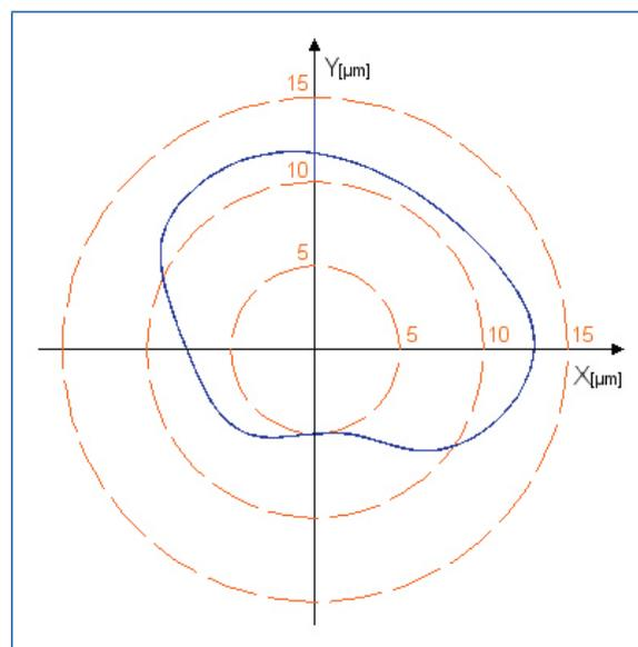
Figure 2. Shaft Orbit: the path of a shaft rotation.
