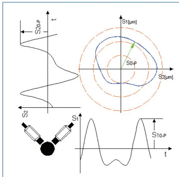
*Figure 6. Shaft vibration So-p max: 0 to Peak Maximum Displacement according to VDI 2059. Two channel measurement of the 0 to Peak Displacement. The S1 and S2 outputs are vector summed to produce a new time series called an “orbit,” which is equal to one shaft rotation. The maximum value of the new time is Smax.*
