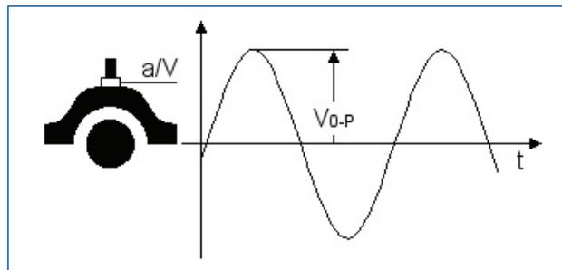
Figure 13. Bearing velocity Peak ( $V_{o-p}$ ): 0 to Peak.
