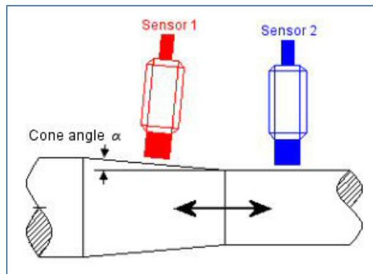
Figure 21. Single-cone measurement set up.
