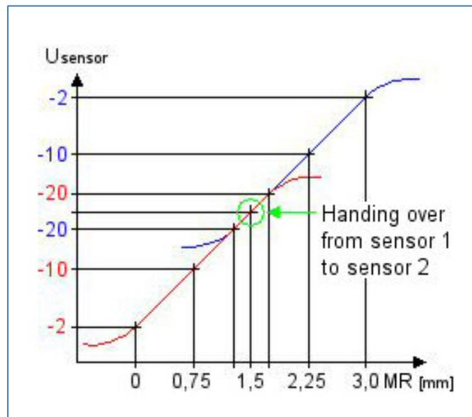
Figure 20. Tandem measurement graph.
