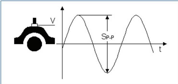
Figure 15. Bearing vibration  $S_{p-p}$ : Peak to Peak.
