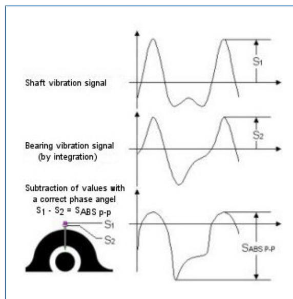
Figure 9. Absolute shaft vibration Sp-p:
