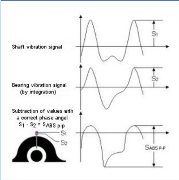
Figure 7. Shaft vibration in Sp-p max: Peak to Peak Displacement according to DIN 45670. Two channel measurement of the peak-peak displacement. A maximum value selection of the two measurements is the result.
