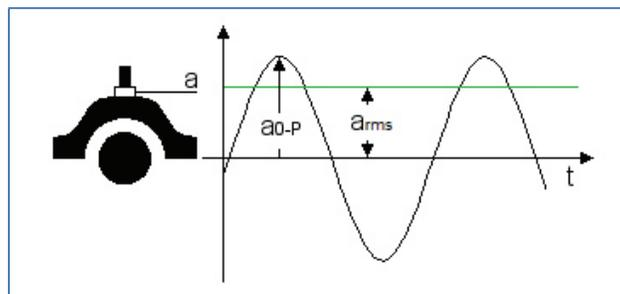
Figure 10. Bearing acceleration RMS ( $a_{rms}$ ): RMS.
