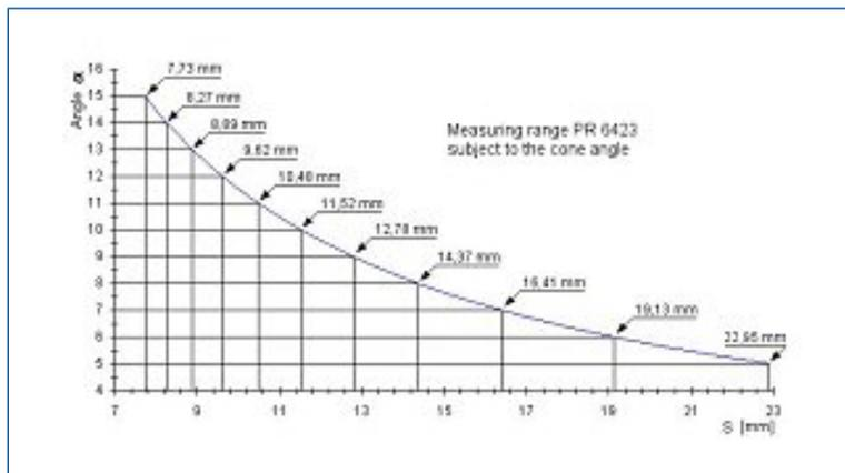
Figure 23. Axial measuring range versus cone angle.
