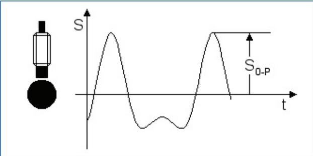
Figure 3. Shaft vibration  $S_{0-p}$ : 0 to Peak Displacement.
