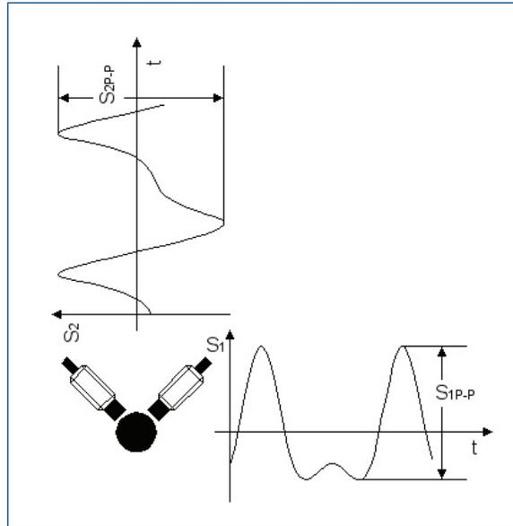
*Figure 5. Shaft vibration Sp-p max: Peak to Peak Displacement according to API 670: Dual-channel peak-peak displacement measurement. The maximum of the two channels is reported as Sp-p max.*
