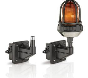
Model LHWB Hazardous Location wall mount bracket is specifically designed for use with Federal Signal's stationary warning lights to provide an easy and consistent means of securely mounting lights throughout a facility. The bracket features a 3/4-inch NPT male pipe connection. Optional bushings are available for 1/2-inch and 1 inch fixture mounting.
