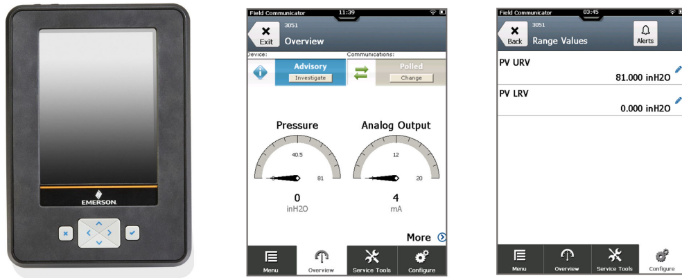
Figure 4-11: After Zero Trim Using Field Communicator
