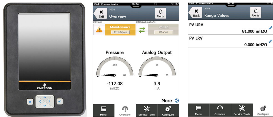
Figure 4-15: Before Re-range Using Field Communicator
