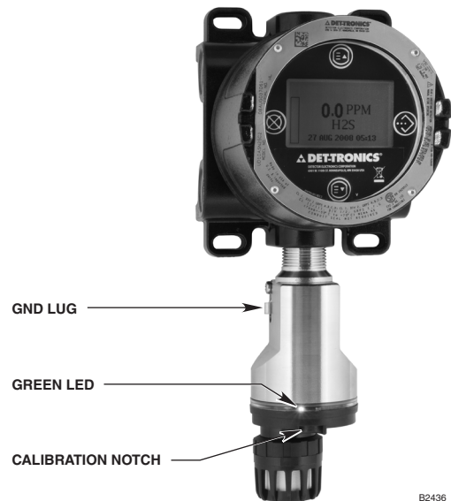
Figure 5—Correct Mounting Orientation for the GT3000
