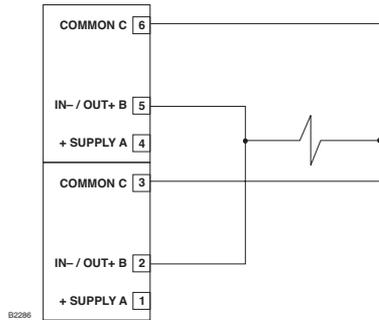
**NOTE: SHUNT/FLYBACK DIODES DO NOT NEED TO BE INSTALLED ON THE FIELD DEVICE. CIRCUIT PROTECTION IS PROVIDED WITHIN THE EDIO MODULE.**
