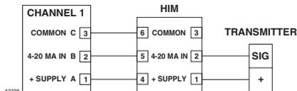
Figure 3-45—Two-Wire Transmitter with HART Interface Module — Non-Isolated 4 to 20 mA Current Output (Sourcing)
