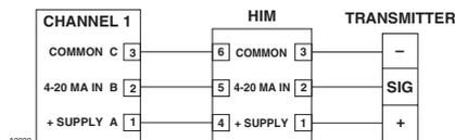
Figure 3-47—Three-Wire Transmitter with HART Interface Module — Non-Isolated 4 to 20 mA Current Output (Sourcing)
