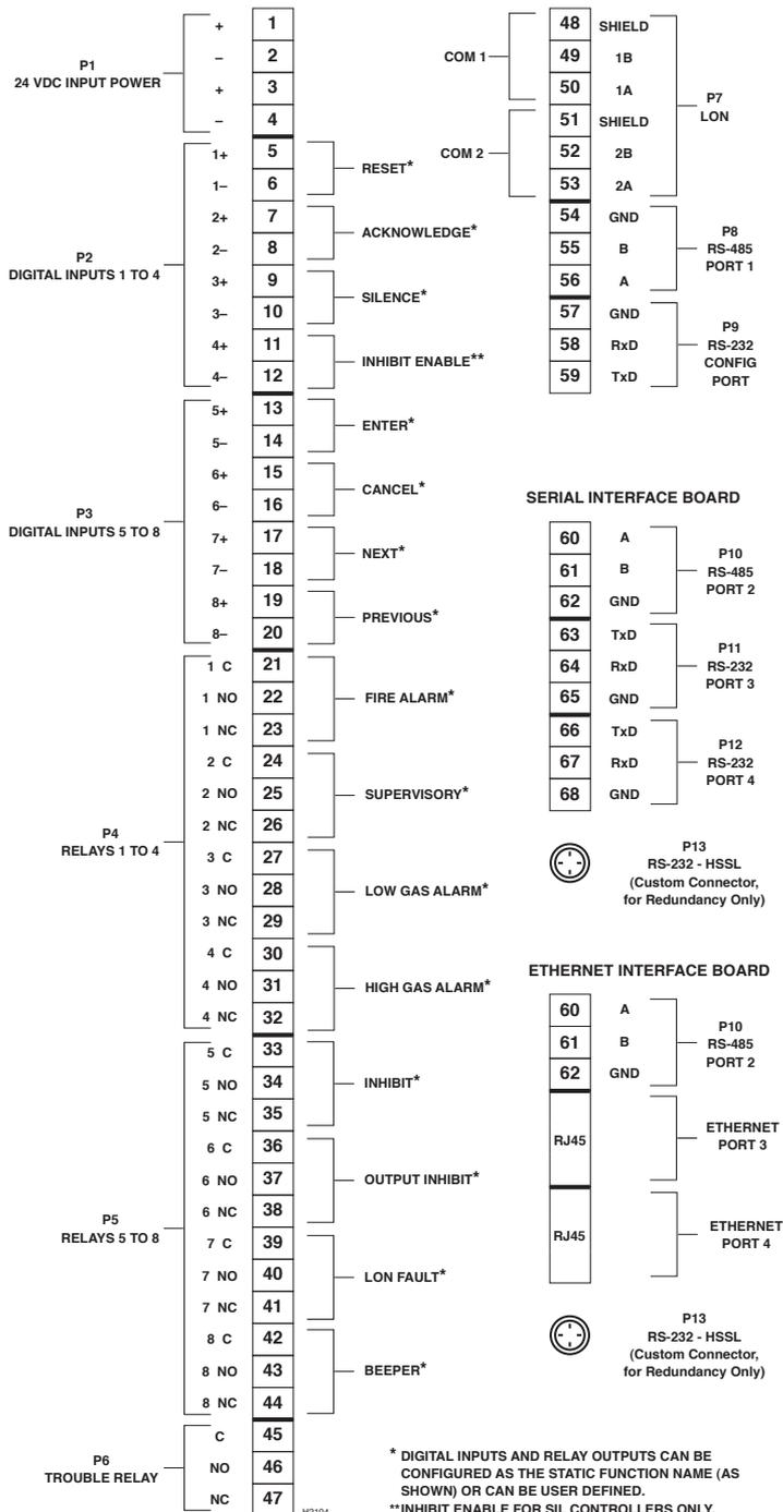
Figure 3-7—EQP Controller Terminal Identification
