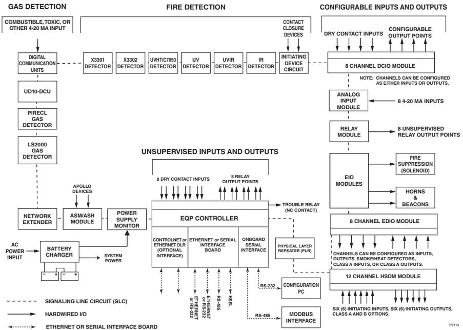
Figure 2-1—Block Diagram of Eagle Quantum Premier System
