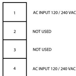
Figure 3-16—J3: AC Input Terminal
