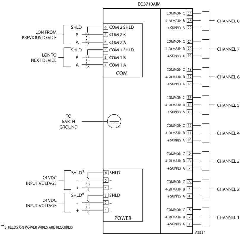
Figure 3-43—Analog Input Module Wiring Terminal Configuration
