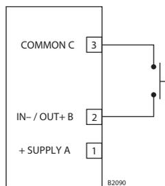
Figure 3-36—Unsupervised Input Configuration
