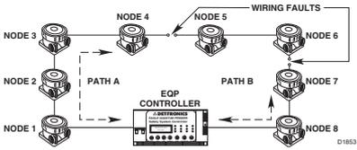
Figure 2-4—Communication over LON with Multiple Wiring Faults
