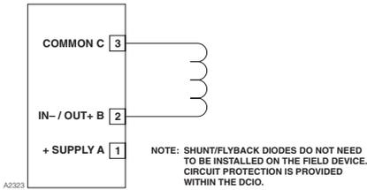
Figure 3-40—Supervised Output Configuration
