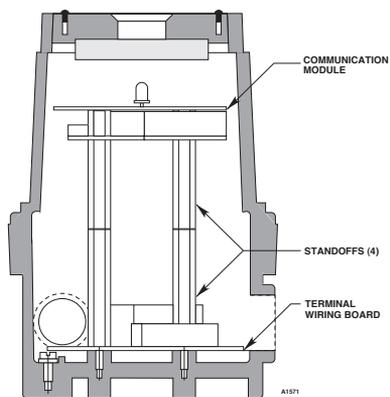
Figure 3-48—Printed Circuit Boards in Universal DCU
