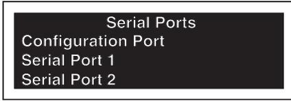
Pressing the NEXT or PREVIOUS pushbutton allows cycling through ports. Pressing the CANCEL pushbutton will return the display to the Main Menu.
