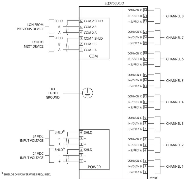
Figure 3-35—DCIO Module Wiring Terminal Configuration
