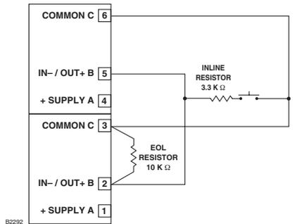
Figure 3-26—Supervised Input Configuration for Opens and Shorts – Class A
