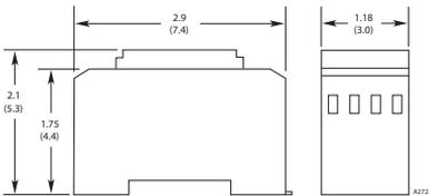
Figure 6-4—Dimensions of EQ2230RSP Module in Inches (CM)
