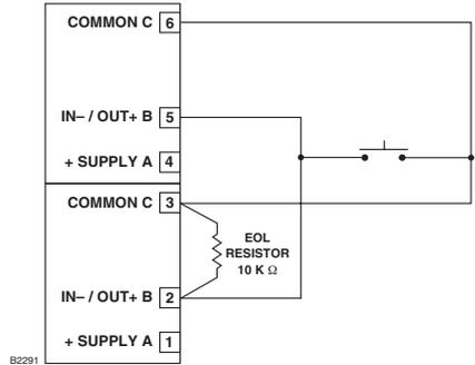
Figure 3-24—Supervised Input Configuration – Class A
