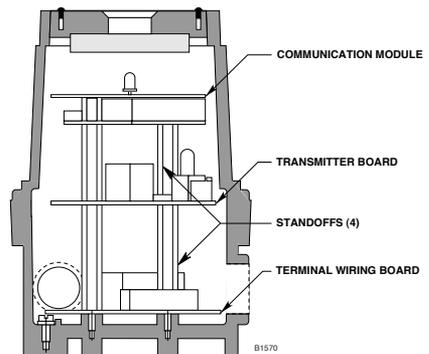
Figure 3-53—Printed Circuit Boards in Combustible Gas DCU
