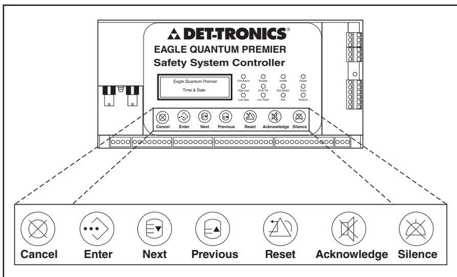
Figure 4-1—EQP Controller Pushbutton Locations
