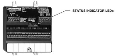
Figure 4-7—DCIO Module Status Indicator Location
