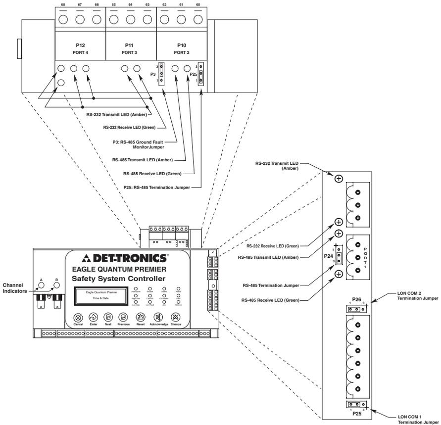
Figure 3-8A—Location of Termination Jumpers, Communication Indicator LEDs, and Communication Ports for Controller with Serial Interface Board
