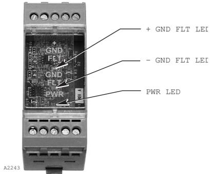
Figure 4-11—Ground Fault Monitor Status Indicator Location
