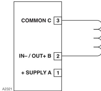
**NOTE: SHUNT/FLYBACK DIODES DO NOT NEED TO BE INSTALLED ON THE FIELD DEVICE. CIRCUIT PROTECTION IS PROVIDED WITHIN THE EDIO MODULE.**
