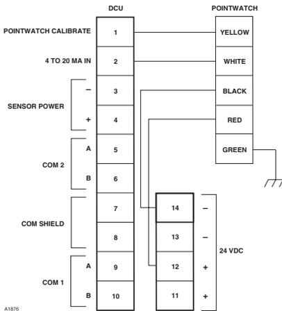
Figure 3-51—PointWatch/DuctWatch Connected to DCU
