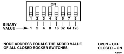
Figure 3-57—Address Switch for DCIO and Relay Module
