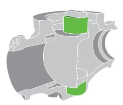
**Reduce service disruptions** with an unbroken coating of ball surface providing a high level of protection on erosive service, and massive trunnions to reduce wear on mechanical parts and preserve packing integrity on high cycle applications. And if maintenance is required, the <sup>2</sup>XC features a true top entry design with minimal parts for rapid in-line maintenance.
