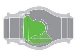
**Run your process for longer** with a double offset C-ball design that enables non rubbing rotation to eliminate wear and extend maintenance intervals. The convex to convex seat is designed to "sweep" particles off the sealing surface without damage, making it ideal for abrasive service which means low wear and long-lasting tight shutoff.
