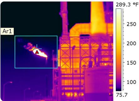
moisture in the air to obtain a good image and relative temperature reading of the flare stack or pilot flame.
