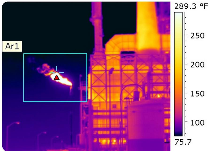
moisture in the air to obtain a good image and relative temperature reading of the flare stack or pilot flame.
