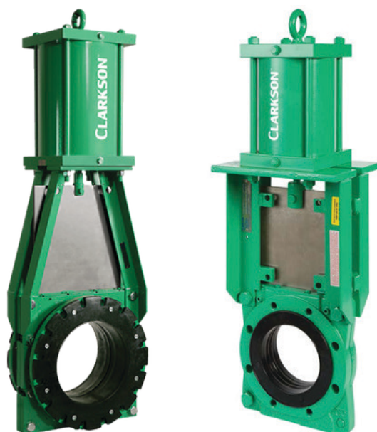
Figure 7: Knife gate valves are common around the flotation and thickener areas. The best valves are tight shutoff, full ported and reversible valves such as the Clarkson™ KGA (left) and the higher pressure rated KGD (right). Both offer zero leakage, replaceable sleeves and handle a range of process pressures.
