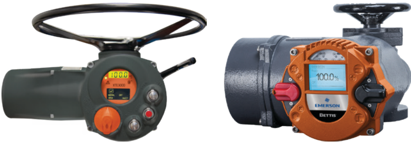
Figure 12: Next-generation electric actuators (Bettis XTE3000 - left) provide SIL 2/3 reliability, programmable stroke profiles, and advanced diagnostics. Other electric actuator designs (Bettis RTS actuator - right) can fail open or closed using a fail-safe spring. Both models provide continuous modulation or on/off service and remote monitoring options.
