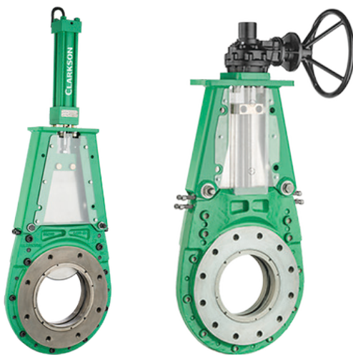
Figure 9: The Clarkson KS1 (left) carries a full 150# flange rating, while the severe service Clarkson KS3 (right) carries a 300# flange rating. Both valves are reversible, have rotatable wear rings, and have advanced seals for excellent shutoff and zero environmental leakage.
