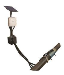
The FSM Area Corrosion Monitor is a non-intrusive solution that can permanently track general and localized metal loss over a pre-defined area in steel pipes, bends and vessels. The multi-pin matrix coverage provides a detailed picture of the pipe area wall thickness, providing a clearer picture of localized corrosion.
