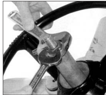
Fig. 5.6 Down Stop two Spanners
