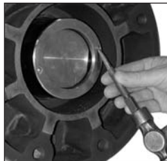
Fig. 4.6 Removal of Retainer
