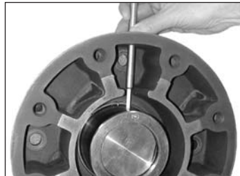
Fig. 4.5 Locating Set Screw
