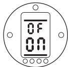
Bus System Positioning Control Screens [ON]
