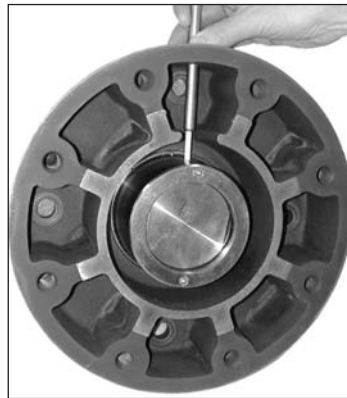
Fig. 4.12 Tightening Retainer Set Screw
