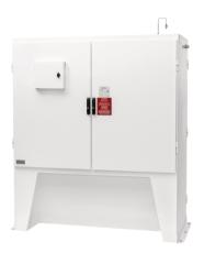
The SpartanPRO™ Surge Relief was developed to meet industry needs. It consists of an electronic pressure controller, color touchscreen HMI, digitally-controlled solenoid valves, a single stage high-pressure letdown regulator, flow metering valves, pressure relief valves, high-pressure nitrogen gas supply cylinders and plenum cylinders. Each are installed within a heated and insulated NEMA 4 cabinet, certified for Class 1, Div 2 / Zone 2 hazardous area locations.
