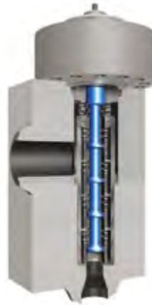
Figure 5.13 Special Valve Design to Eliminate Cavitation
