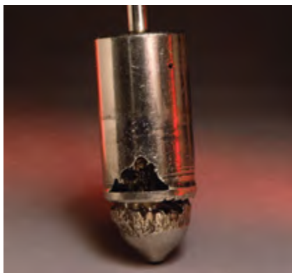
Figure 5.8 Typical Appearance of Flashing Damage
