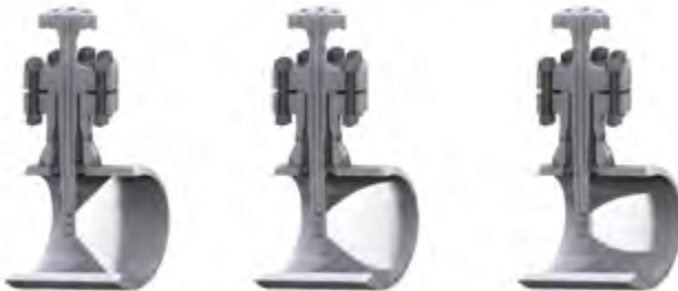
Figure 7.3 Desuperheater Spray Penetration
