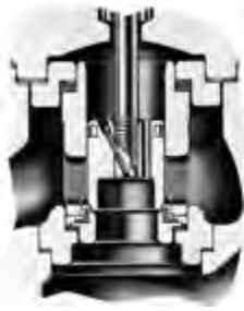
Figure 3.36 Adapter Method for Providing Reduced Flow Capacity
