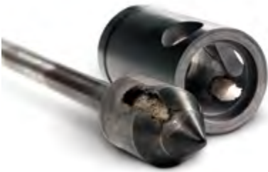
Figure 5.9 Typical Appearance of Cavitation Damage
