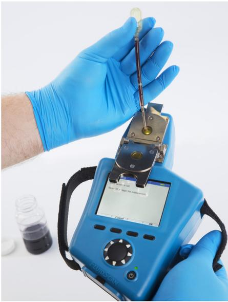
Patented flip top cell for accurate, easy sampling
