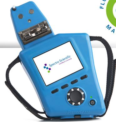
The FluidScan 1000 Series provides quantitative measurement of a lubricant's condition and plays an important role in predictive maintenance. Using the device, you can eliminate unnecessary oil changes or service by testing not just servicing the oil.
