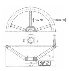
This Handwheel is the type using air impact wrench and if can be made properly according to customer's request.
