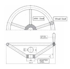
If there is no request from customers, we will make handwheel as per the above table. As option, the material can be changed and Handwheel size can be suitable for all model.
