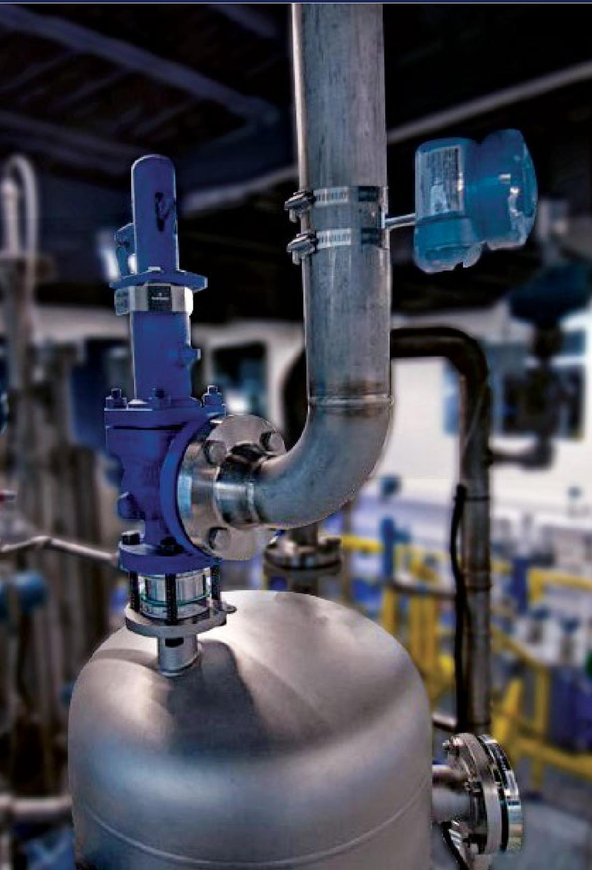
The challenge is identifying which valves are not working correctly. If operators want to know what is happening with a particular PRV, they typically rely on local inspection, or they monitor normal process pressure measurements for indication of operation near the PRV's setpoint.
