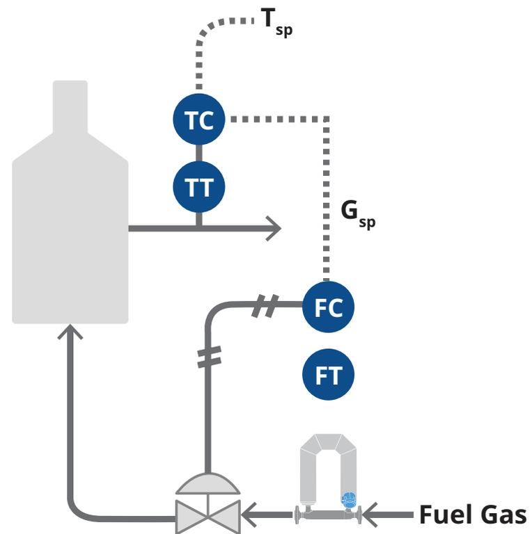
Figure 1.4: Fuel flow measured in pounds or kilograms per hour makes it much easier determine optimal stoichiometric air flow.
