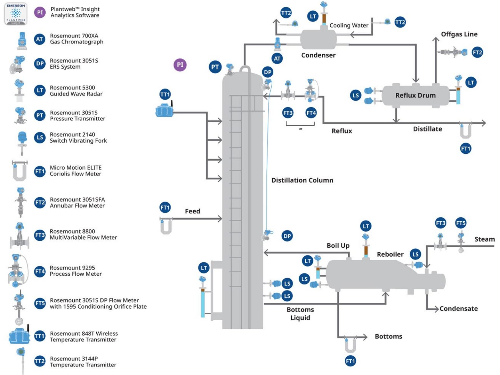
Figure 6.1: Distillation columns and their associated equipment can cause a wide range of problems, resulting in high costs and low-quality products.
