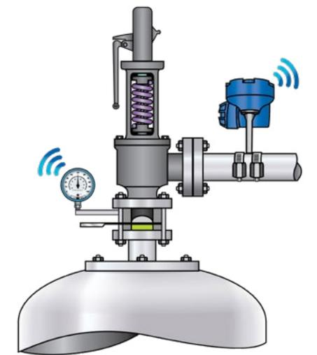
*Figure 4.4: Mounting a Rosemount 708 Wireless Acoustic instrument on the discharge pipe of a PRV detects when release incidents happen, and if leakage continues due to an incomplete seal. No process penetration or shutdown is necessary for mounting.*
