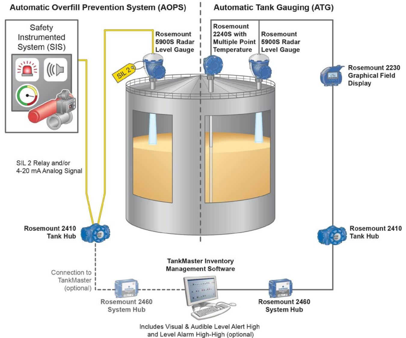
Figure 7.2: Level instruments for safety and control must function separately, even when monitoring the same tank.
