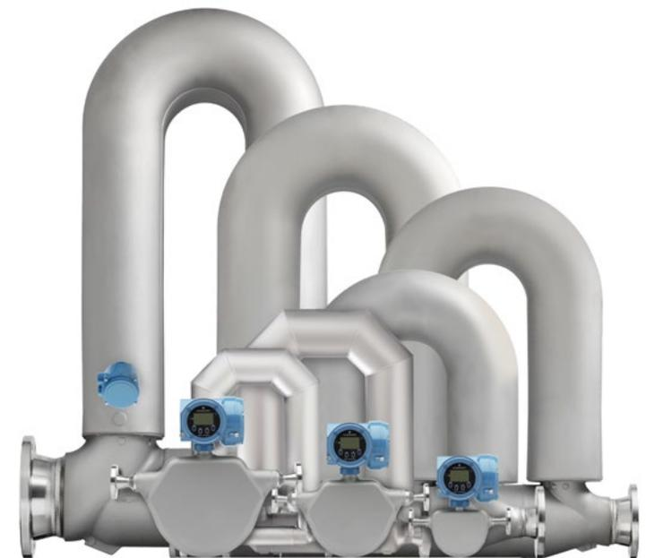
*Figure 1.5: Micro Motion Coriolis flow meters measure mass natively, so there is no need to make a correction when density changes.*
