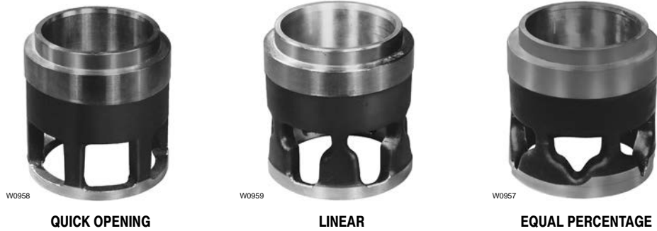
Figure 1-28. Characterized Cages for Globe-Style Valve Bodies
