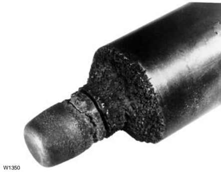
W1350 Figure 4-3. Typical Cavitation Damage
