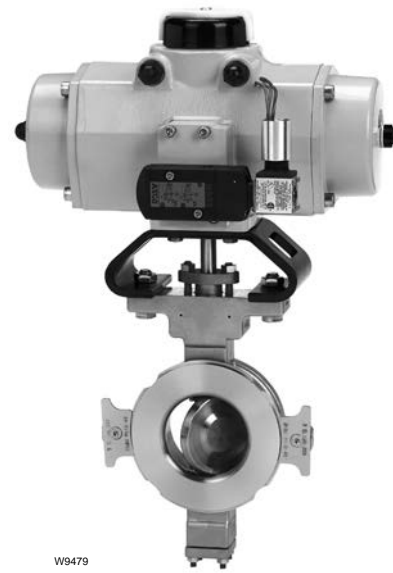
Figure 2-7. The FieldQ™ actuator is a quarter turn pneumatic rack and pinion actuator. It comes with an integrated module combining the solenoid and switchbox into a low profile, compact package.
