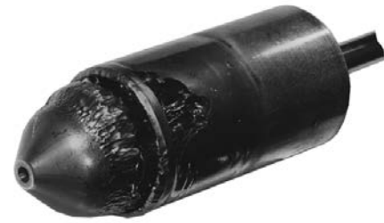
Figure 4-6. Typical Flashing Damage
