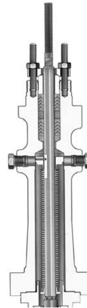
Figure 1-18. ENVIRO-SEAL™ Bellows Seal Bonnet
