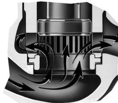
Figure 6-1. Whisper Trim I cage used for reducing aerodynamic noise
