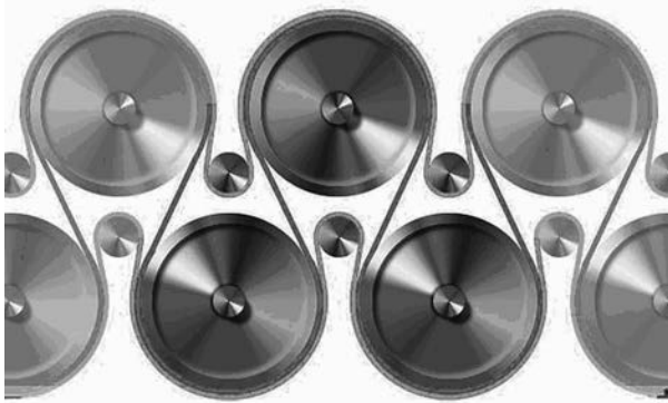
Figure 17-16. Two-Tier Drying System
