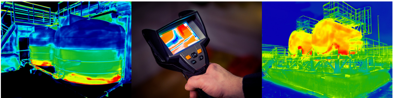
Figure 1. FTIR camera being deployed for leakage detection in storage tanks
