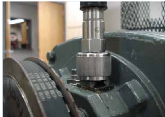
Typical magnetic mounting of accelerometer
