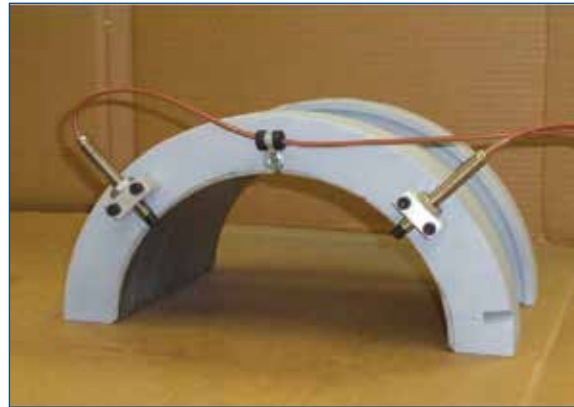
Typical displacement probe mounting on a large sleeve bearing
