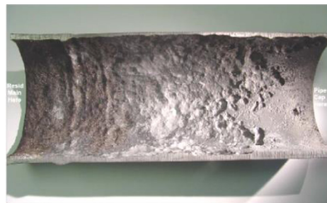
Figure 4: Naphthenic acid corrosion [courtesy of Nalco Champion]
